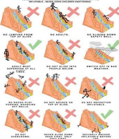
We advise only 2 users at a time. It is strongly advised to have 2 operators supervising this equipment, one at the platform top and one at the bottom. Ensure you have adequate anchorage. Measurements and calculations for this can be found in pren en 14960 on our site right hand side.
